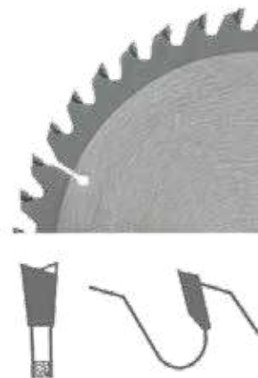
ATB teeth alternate upper bevel
