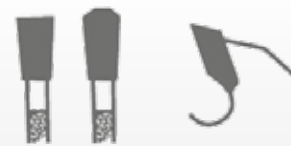
TCG teeth disc upper alternating bevel for laminated wood cutting.
