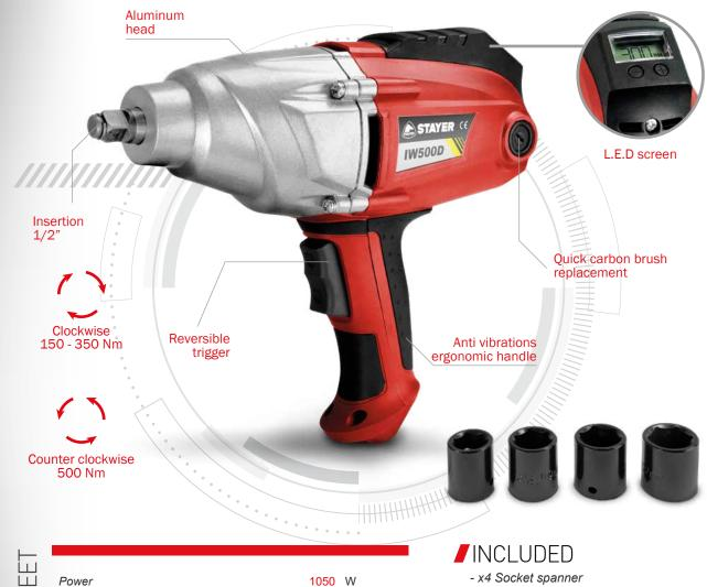
Power 1050 W No load speed 0-2200 min-1 Tightening torque 150-350 / 500 Nm Insertion 1/2" UNF 3.5 kg Weight
