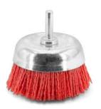
Brushes made of nylon filaments with aluminum oxide abrasive grains. It does not scratch or alter the dimensions of the pieces. Ø75mm Coarse grain.
