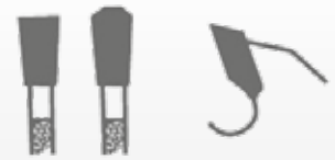
TCG teeth disc upper alternating bevel for laminated wood cutting.
